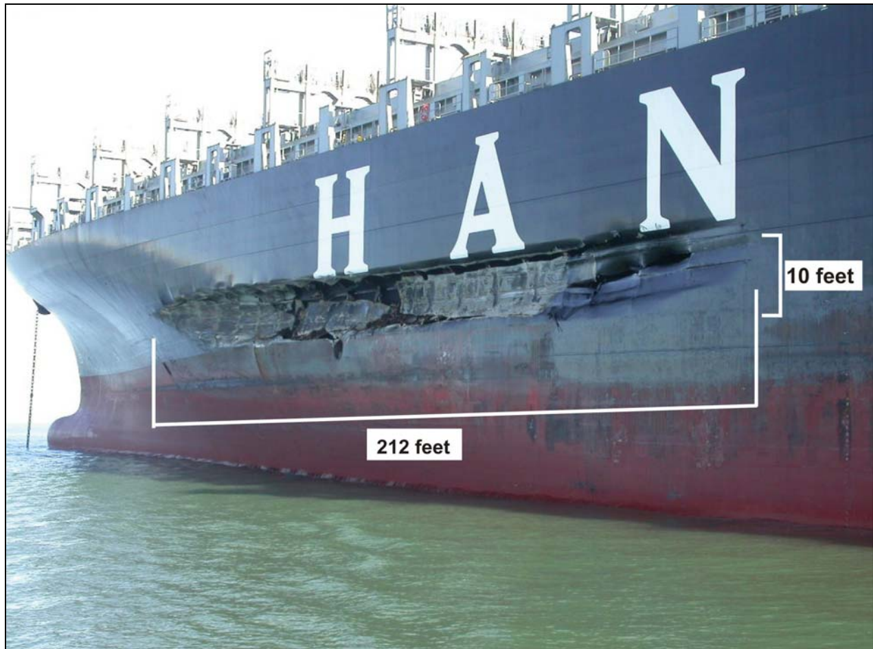
Figure 4. Damage to the forward port side of the Cosco Busan after the allision with the bridge tower.
